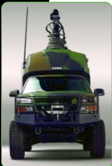
GM's hybrid military Silverado comes equipped with a fuel cell for silent auxiliary power.
